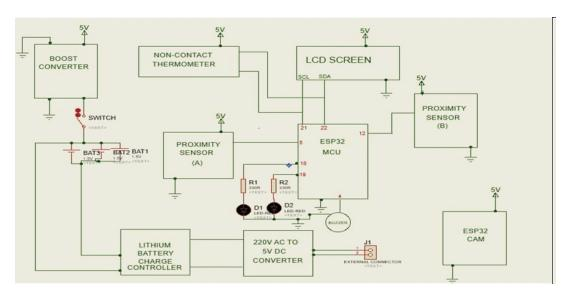
Figure 1: Circuit diagram of the proposed System
